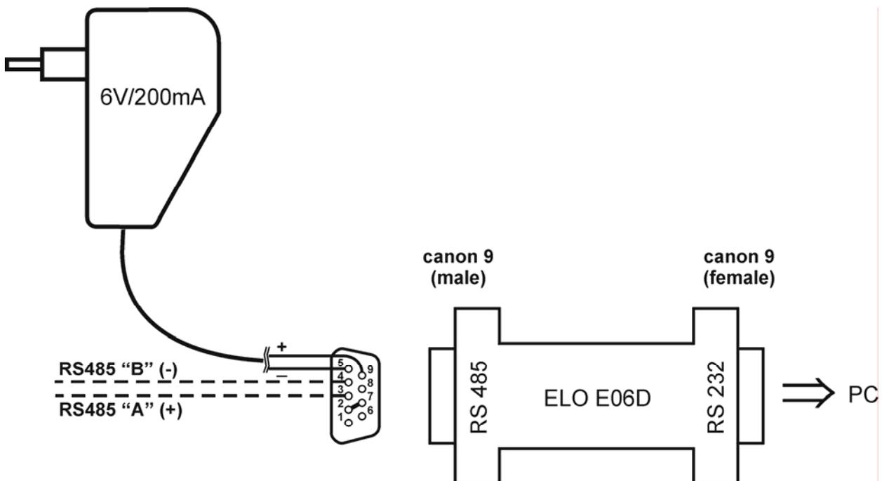
The ELO E06D converter is an optional accessory for connection of transmitter/transmitters with RS485 interface to the PC via serial port RS232. Connect connector marked RS232 directly to the PC, connect power to connector marked RS485. Power voltage **+6V DC** from an external acdc adapter connect to **pin 9**, **0V** connect to **pin 5**. Also mutually connect pin 2 and pin 7. Link RS485 is connected across **pin 3 (A+)** and **pin 4 (B-)**.
