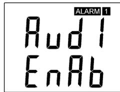
**Acoustic alarm assign to relay 2**
